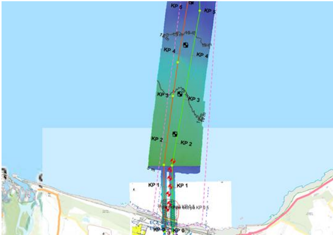
Fig 2 Backhoe trenching routes.
