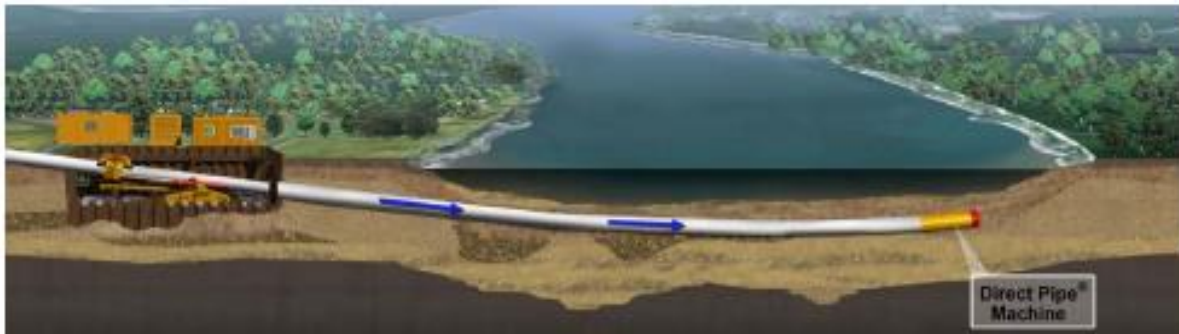
Fig 6. Micro tunnelling machine
