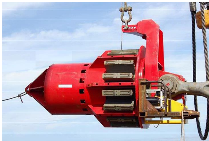
Fig 9 ILT – Internal pile Lifting Tool – used to stab and lift piles
