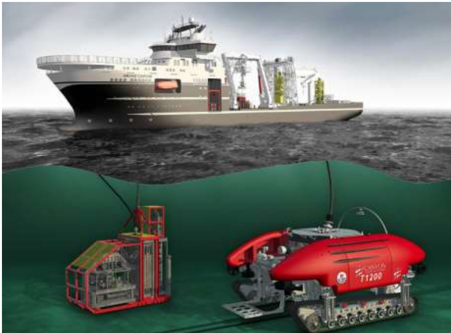
Fig. 2 Grand Canyon Tracked Trenching System
