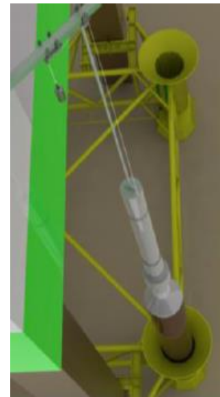
Figure 6 - Hammer Positioned on Pile
