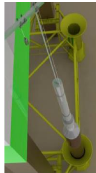
Figure 8 - Hammer Positioned on Pile
