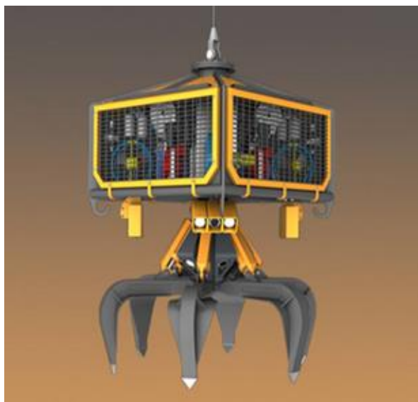
Fig 4 - UTROV Grabber System for Boulder Removal
